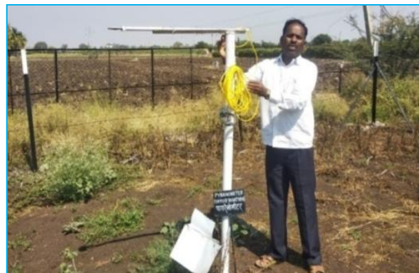
Net Radiometer installed at AET Rahuri
