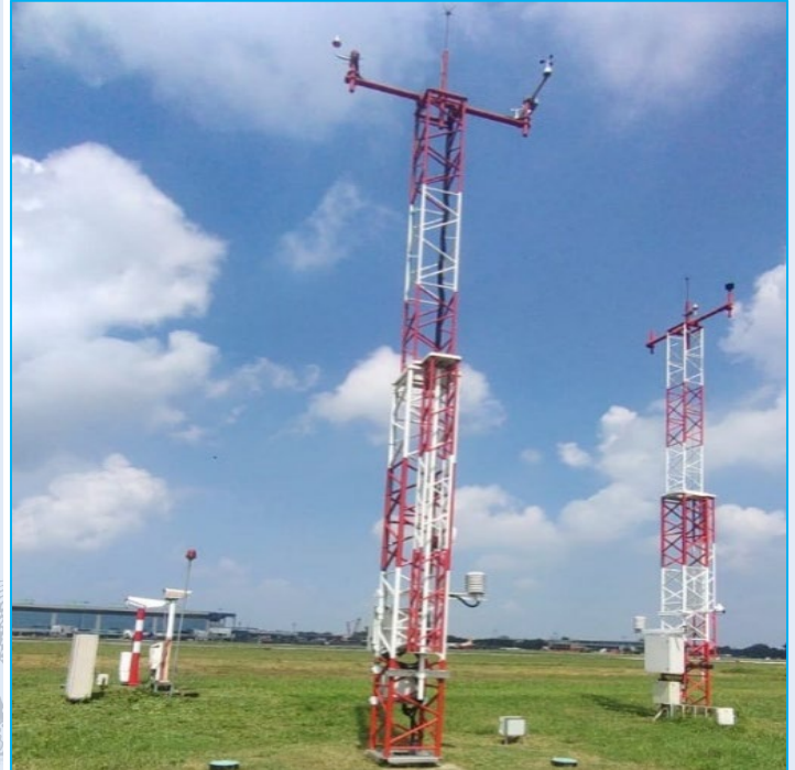
Mast of Automated Weather Observing System (AWOS) (Carrying Wind Sensor, ATRH Sensor and Pressure Sensor)
