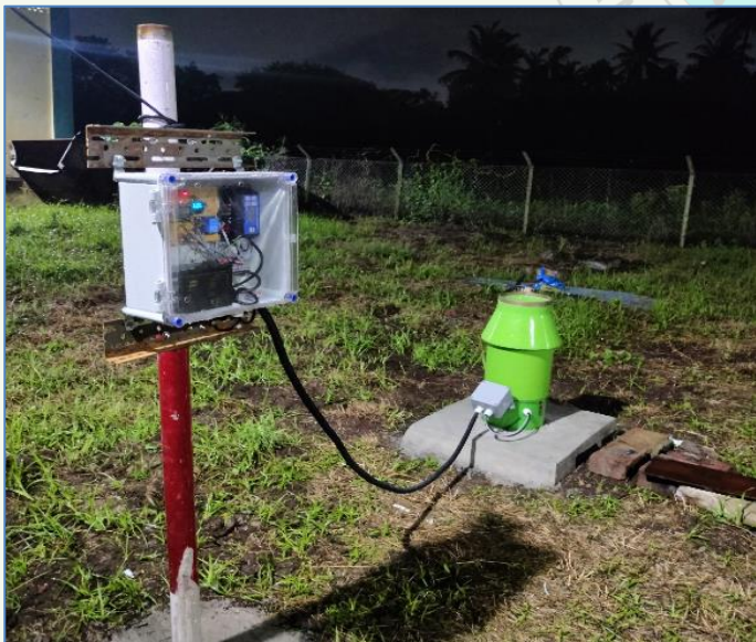
In house developed Rain gauge installed at CAgMO Surface Observatory on experimental basis
