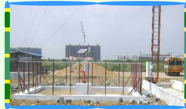
Automatic Rain Gauge at Sathyabama University
