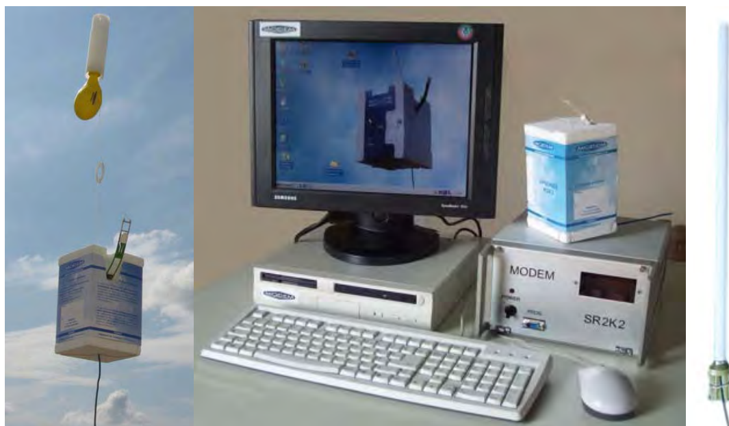
Fig. 2. Ground System with Receiver & Processor
