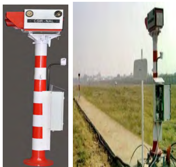
Fig. 7.1. Drishti at IGI Airport and Main Sensor (Transmitter & receiver unit)
