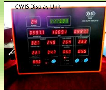
Fig. 12. CWIS, CWIS System Data Logger and CWIS Display Unit
