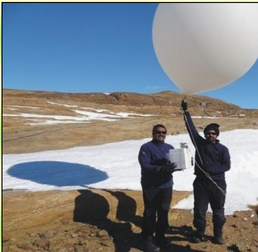
Fig. 17. Ozonesonde ascent at Bharati, Antarctica
