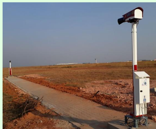
Fig. 9. DRISHTI system installed at Kolkata airport
