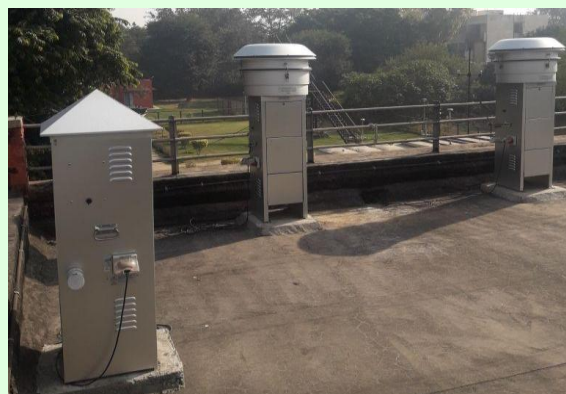
Fig. 6. High volume sampler for collecting PM 10 , PM 2.5 and Total Suspended Particulate Matter
