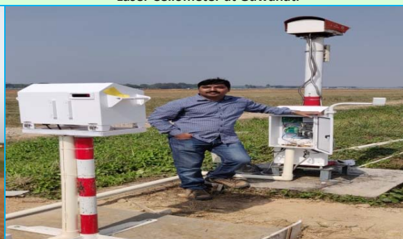
Fig. 4. DIWE System at Hissar and Laser Ceilometer at Guwahati
