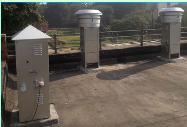
Fig. 10. High volume sampler for collecting PM 10 , PM 2.5 and Total Suspended Particulate Matter
