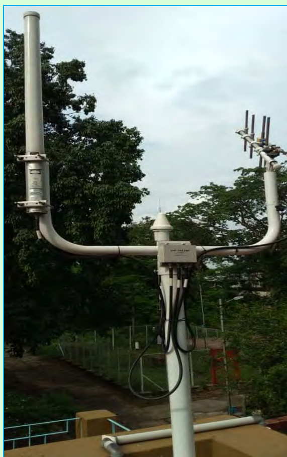
Fig. 3. Radiosonde antenna installation at RS/RW Bankura, West Bengal
