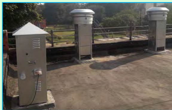
Fig. 27. High volume sampler for collecting PM 10 , PM 2.5 and Total Suspended Particulate Matter
