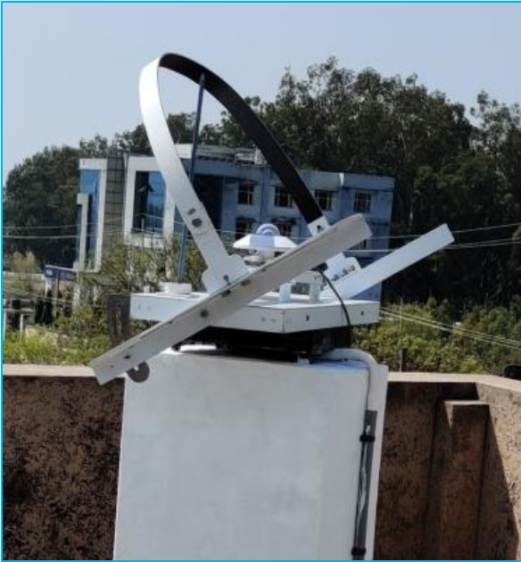
Fig. 7. Pyranometer for measurement of diffuse radiation
