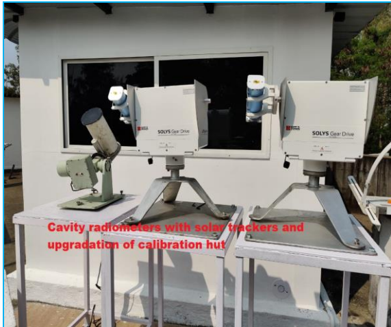
Fig. 8. Cavity radiometers with solar trackers and upgradation of calibration
