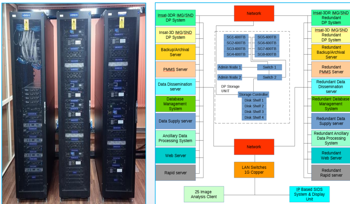
Fig. 27. Block diagram of MMDRPS system
