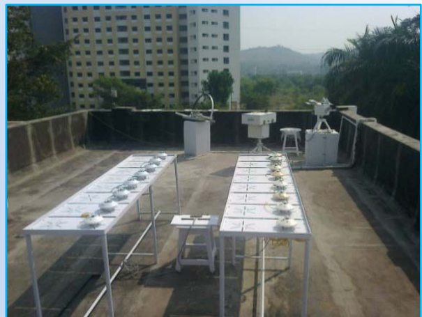
HF Cavity radiometer and PMO6 facility (a reference instrument) to measure Direct solar irradiance.
