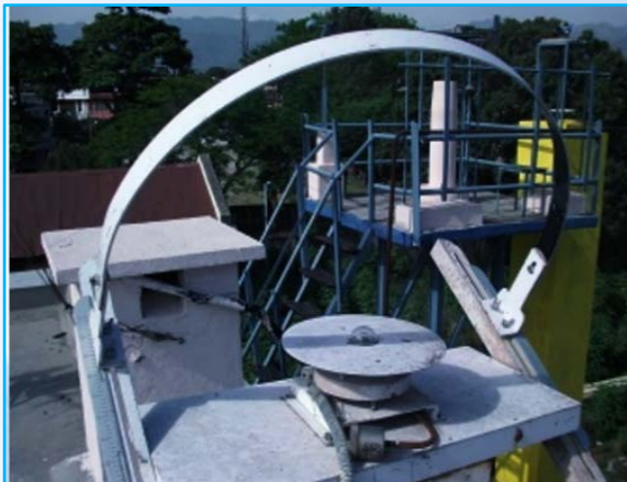
Thermoelectric Pyranometer with shading ring (Measure Diffuse Solar Radiation)
