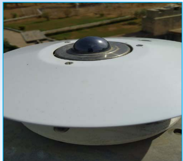
Pyrometer (Precision Infrared) (Measure Terrestrial Radiation)
