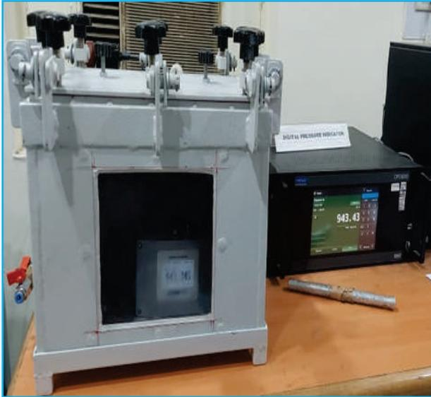
**Fig. 12. In-House manufacture pressure chamber**
