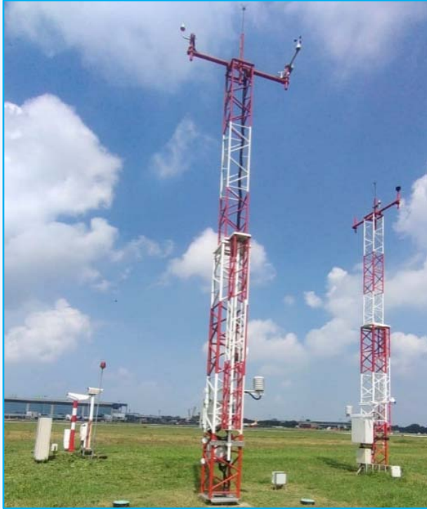
Fig. 6. Mast of Automated Weather Observing System (AWOS) (Carrying Wind Sensor, ATRH Sensor and Pressure Sensor)
