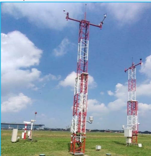
Mast of Automated Weather Observing System (AWOS) (Carrying Wind Sensor, ATRH Sensor and Pressure Sensor)
